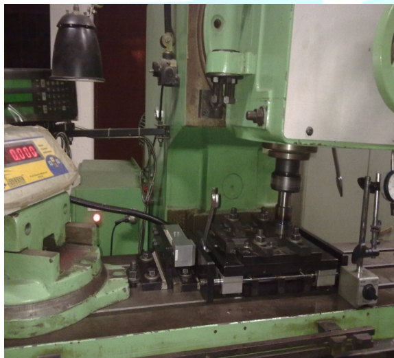
Fig. 2. Experimental setup of FSW
