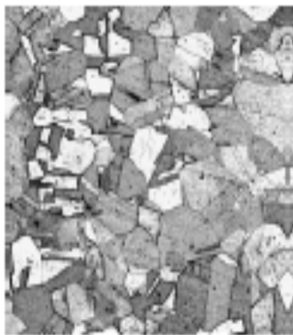
Fig.11. Microstructure of pure copper
